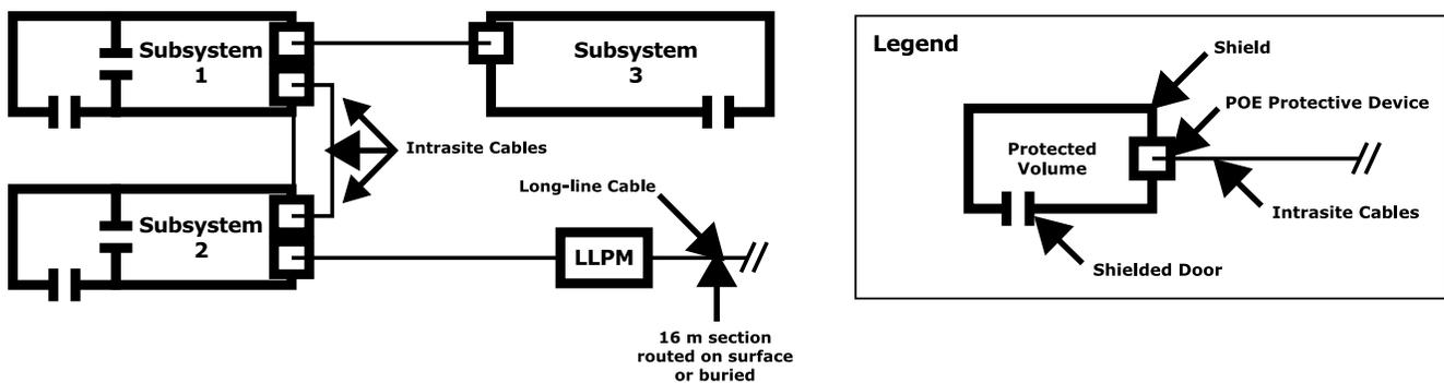
Figure 1: The basic premise of shielded enclosures and screened environments is to create “Faraday Cages” at each separate subsystem with filters applied at all point of entry (POE) for cable runs between enclosed regions.
